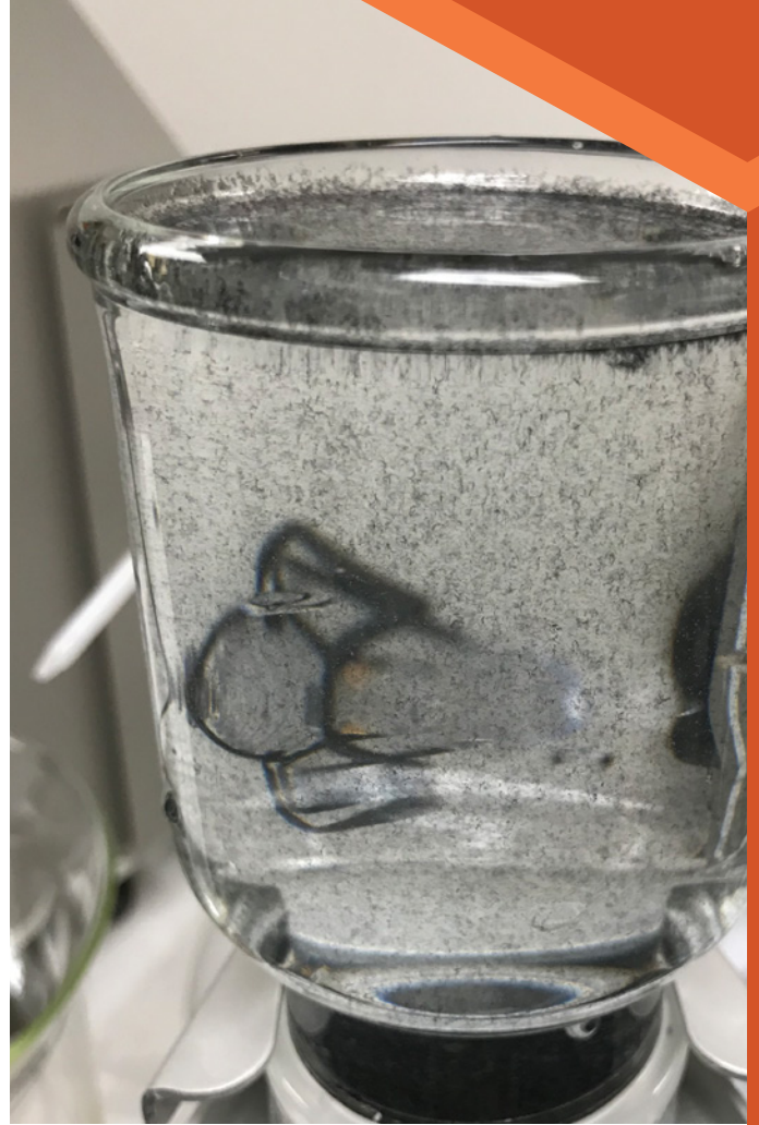
Suspended fibers in water in vacuum filtration funnel. CREDIT: HEATHER ELLIOT
